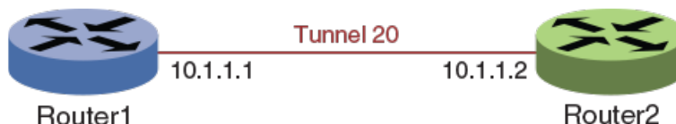
FIGURE 16 Deployment of IPsec Using the Default Settings
